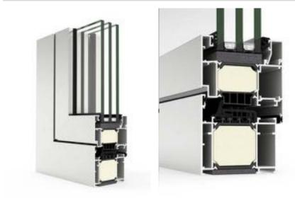
This european groove hinged system allows to achieve maximum levels of water tightness, energy efficiency and acoustic protection with less fabrication and installation time. With 80 mm of frame depth, it is suita-ble for the most severe climate conditions, with unbeatable energy efficiency rating.
